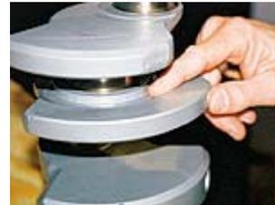
The logic here is easy enough to understand--there is such a wide selection of small-block Chevy rods on the market today, trimming the mains down to size pays for itself in being able to get off-the-shelf connecting rods. The final stroke length is 3.475 inches, resulting in a 365-cube displacement when teamed with the 4.087-inch bore. The crankshaft counterweights were
