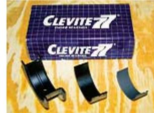
All of the engine bearings are Clevite 77 parts--and more PolyDyn coatings can be found here, as well. This time, the material is PolyDyn DL--another dry film lubricant that oil sticks to. If there is a starvation problem, the coating is designed to keep the bearings from sticking to the journal. Oiling holes will be drilled to each specific main bearing after the trial assembly period. DMR likes to see .0030- to .0035-inch clearances on the main bearings and .0025-inch clearances on the rods.
