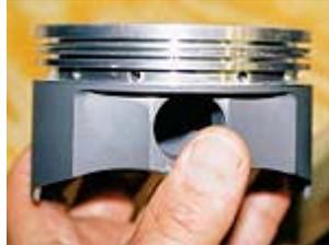
The coating also reflects heat back into the combustion chamber for a more complete burn of the mixture, allowing more power with less ignition timing. The piston skirts are coated with a material called PolyDyn RP, a high-pressure, dry film lubricant, unique in that oil gets it wet. This will protect both the piston skirt from galling and the cylinder walls from scuffing.
