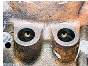
The lifter bore oiling holes are also restricted, this time down to a tiny .040-inch hole. That's still plenty of oil to lubricate the lifters, but limiting oil flow to the top end is the key. How small are these restrictors?
