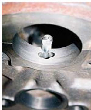
The next step in oil control is to use these main bearing galley restrictors. Limited to a .125-inch hole, they keep precious oil in the bottom end of the engine. Enough lubricant finds its way to the top end to keep the valvetrain happy but can starve the mains without these restrictors in place. These are not too difficult to install.
