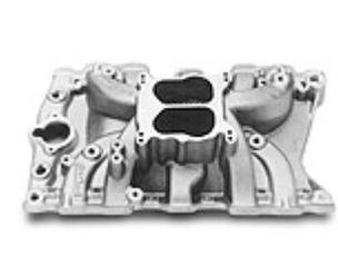
The intake manifold will be an Edelbrock Performer RPM Olds 350 (PN 7111). This will be modified along with the heads to create a matched performance package for power between 2,500-6,500 rpm.
