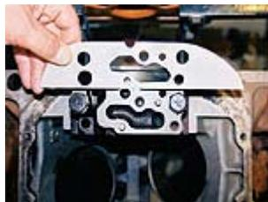
The first step is to match and port the oil pump housing and pump boss. This DMR-built oil deflector is used as a template for both the block-side pump boss and the pump casting itself.
