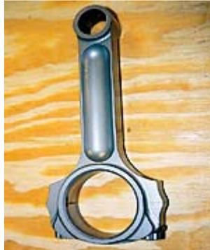
The rods connecting the pistons to the cranks are forged small-block Chevy units from Oliver. They measure in at 6.2 inches in length, and weigh 660 grams. Pin diameter is .927 inch (small-block Chevy OEM diameter), and the big ends are finished in factory SBC 2-inch diameters. Like the crankshaft counterweights, the connecting rods are coated with PolyDyn PD-14 Silver, an oil-shedding coating that will not allow oil to stick to the parts. This reduces
