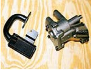
More oiling system information! The oil pump is an out-of-the-box unmodified Melling HV pump (PN M22FHV). Dick has used plenty of these pumps with no problems. The 7-quart oil pan and matching pickup are Moroso parts, but DMR prefers to sell the pan, pickup, and pump as a complete package under PN DMR 20482-5.
